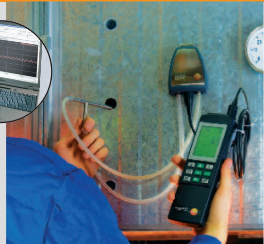
Pitot tube measurement with external 100 Pa probe
